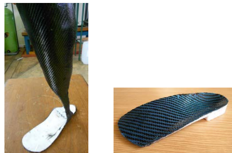
Figure 2. Sample AFO with ABS core and carbon fibre reinforcement (left) and PLA+carbon fibre (right)
