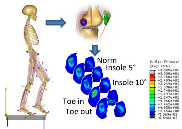
Figure 1: Scheme of the multiscale simulation: (left, top) personalized musculoskeletal model; (right, bottom) results of personalized FE models, showing maximum principal stress patterns at the medial cartilage for each configuration for the second axial peak force of gait.
