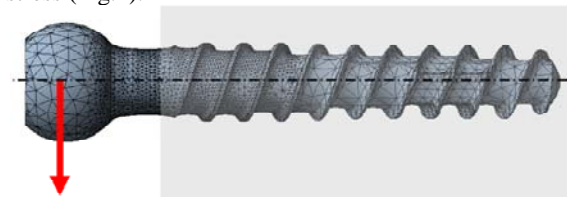
Figure 1: FEA model used for stress optimization
