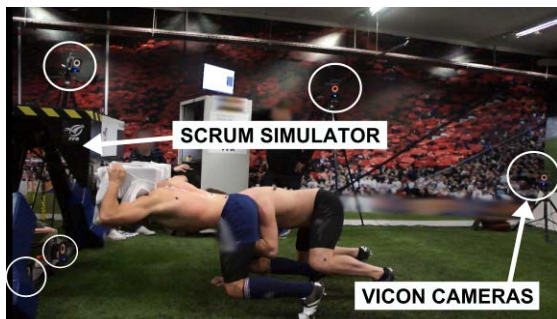
Figure 1: Subjects, Vicon cameras and scrum simulator positions during the tests.
