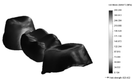
Figure 2. Stresses in dental crown
